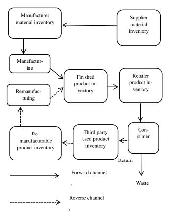
Fig. 1: Model for direct manufacturing and remanufacturing
