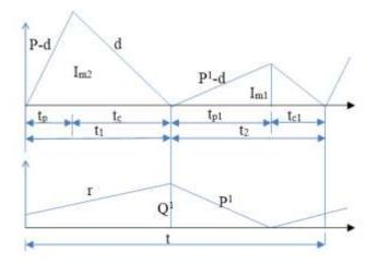
Fig. 2: Inventory model for direct manufacturing and remanufacturing
