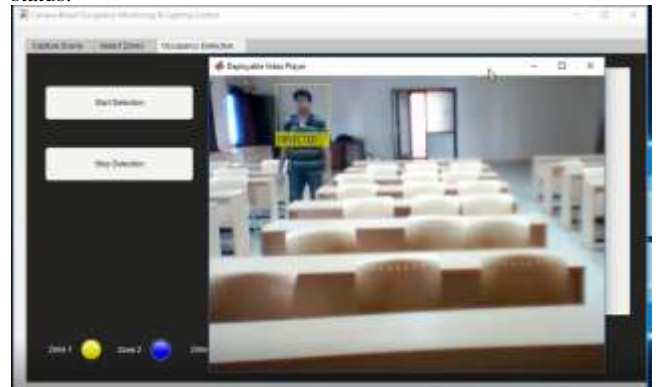
Fig. 6: Snapshot of graphical user interface tracking person in the left side zone
