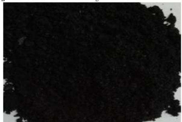
Fig. 8: Crushed carbon grinded completely to develop into activated carbon.
