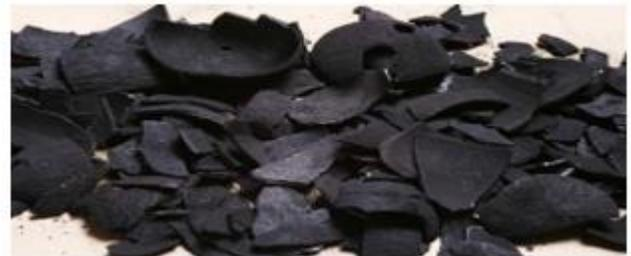
Fig. 7: Dried shells was burnt under high flame to become crushed carbon.
