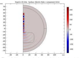
Figure.2. Wave propagation from the dielectric rod plotted with E
