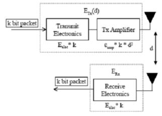
Fig. 2: Radio Model of a Wireless Device
