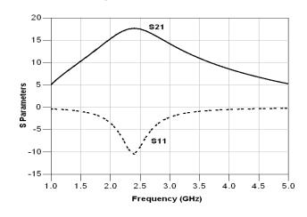
Fig.2 S - Parameters The noise figure (NF) value of 1.1 dB is obtained as shown in Fig.3.
