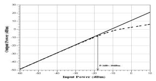
intercept point is the extrapolated intersection of desired output and third order intermodulation (IM) output as a function of input RF level. The obtained IIP3 value is +5 dBm .
