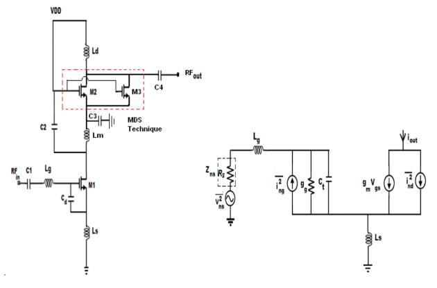
Fig.1(a) Schematic of Current Reuse LNA with MDS (b) Small Signal Equivalent Circuit of input stage
