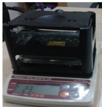
Fig.2: Densimeter used to measure the purity of gold
