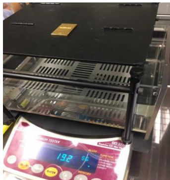
Fig.9: Calibration of the densimeter using NMIM's standard gold
