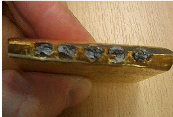
Fig.1: 100 g gold bar plated with tungsten
