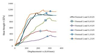
Fig. 4: Shear Strength vs Displacement Residual Condition
