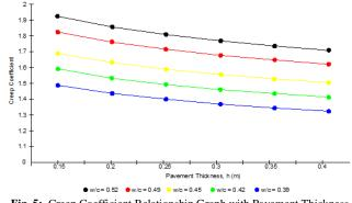
Fig. 5: Creep Coefficient Relationship Graph with Pavement Thickness
