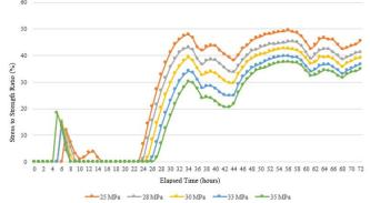
Fig. 10 : The relationship between the start time and the stress - strength ratio of concrete (%) for various concrete (fc ') and nighttime construction, subgrade of soil reaction (k) 27 MPa / m, thick (h) 25 cm and length (L) 3.44 m
