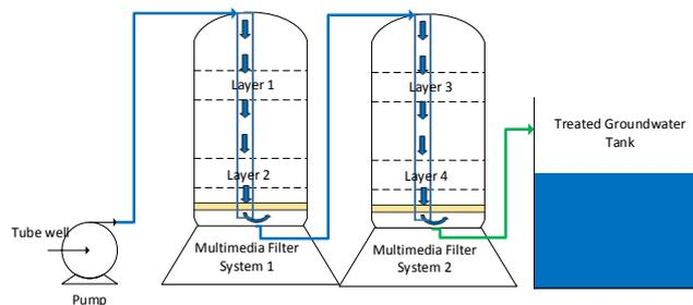
Fig. 3: Groundwater flow treatment in multimedia filter system
