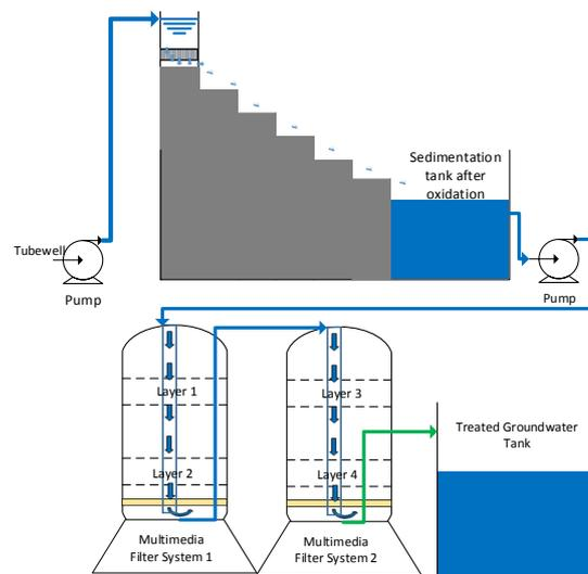
Fig. 7: Integrated between stepped cascade aeration and multimedia filter system
