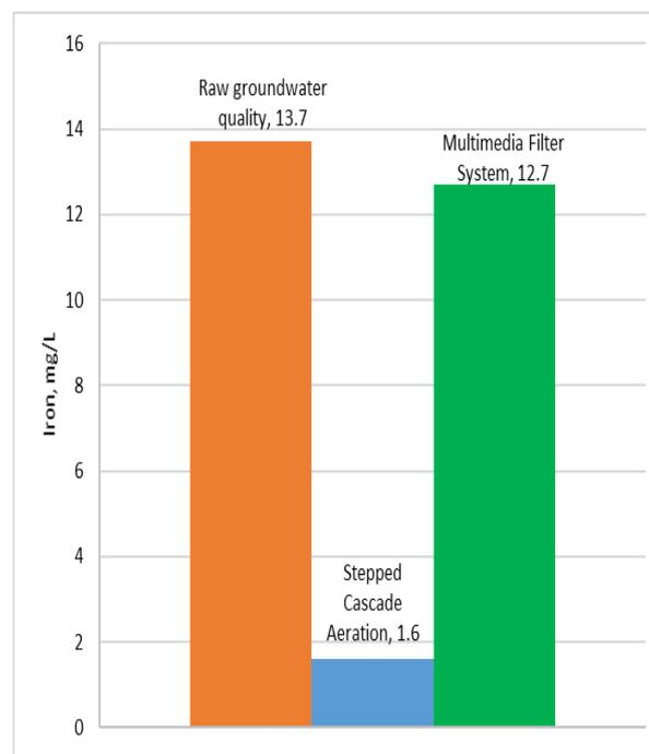
**Fig. 6:** Comparison removal iron between stepped cascade aeration and multimedia filter system from raw groundwater
