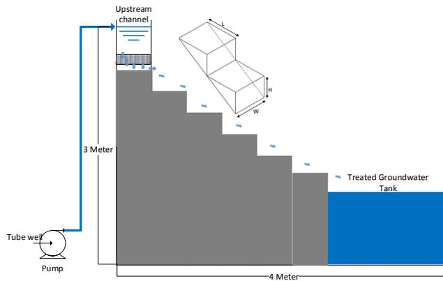
Fig. 1: Stepped cascade aeration design
