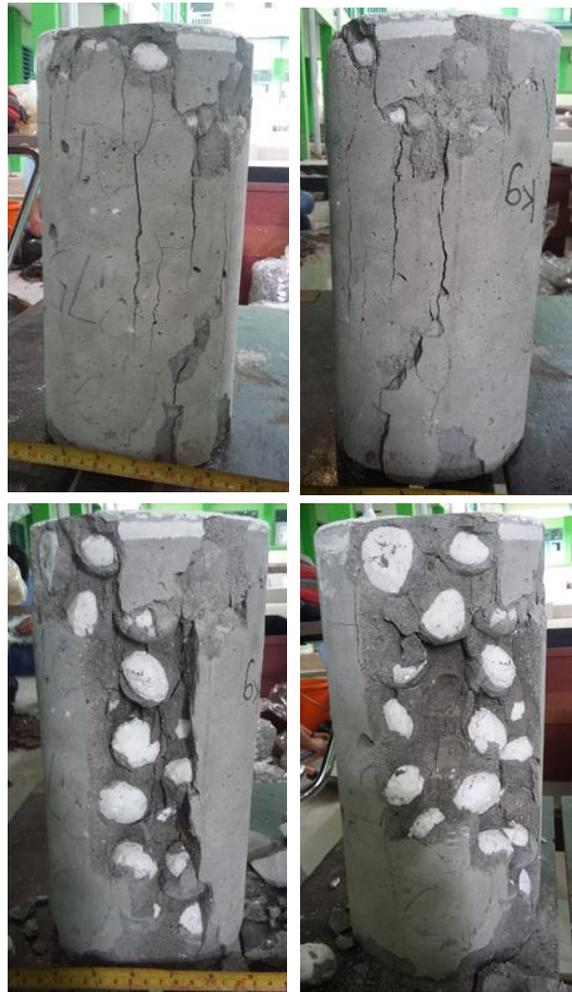
Fig. 6: Collapse pattern of concrete and deployment of aggregate StyM100%
