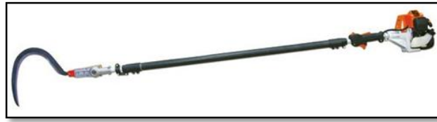
Fig. 1: A motorised cutter for oil palm harvesting - Cantas R
