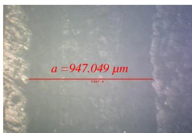
Fig. 14: Wear track width composition 60 wt. % filler and 40 wt. % matrix (zoom 50 X).
