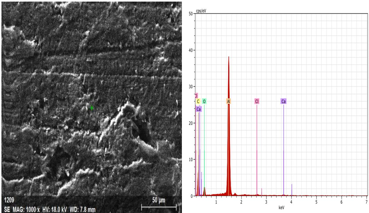
Fig. 25: SEM/EDS Microstructure of developed brake pad with 70 wt. % filler and 30 wt. % matrix
