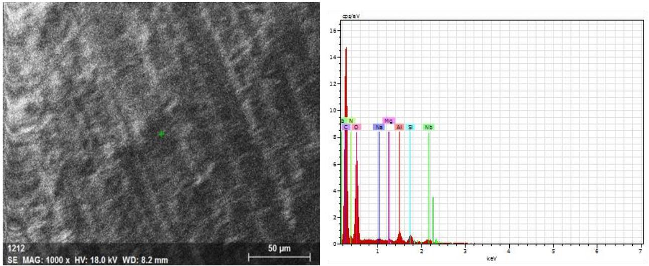
Fig. 23: SEM/EDS Microstructure of brake pad with 50 wt. % filler and 50 wt. % matrix.
