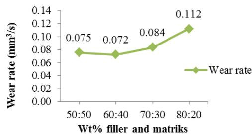
Fig. 21: Variation of wear rate with % filler and matrix weight
