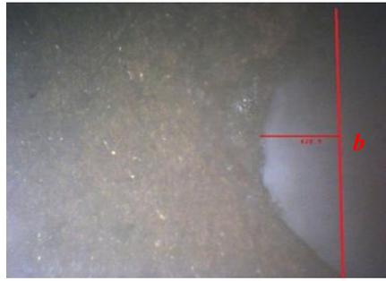
Fig. 19: Wear track depth composition 70 wt. % filler and 30 wt. % matrix (zoom 50 X)
