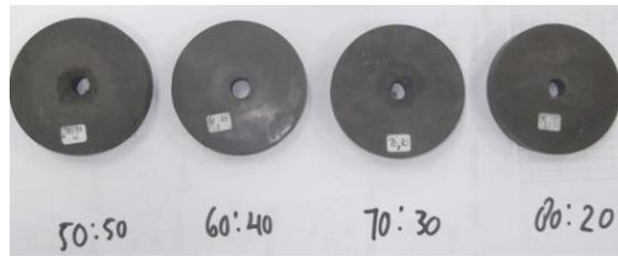
**Fig. 8:** Specimens of drum brake pad materials before wear test
