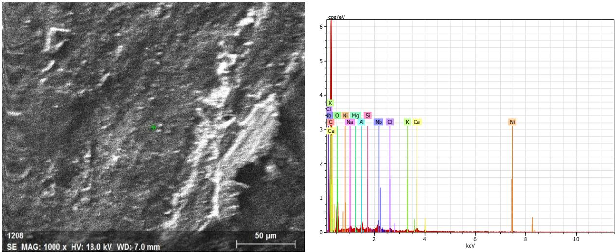
Fig. 24: SEM/EDS Microstructure of developed brake pad with 60 wt. % filler and 40 wt. % matrix.
