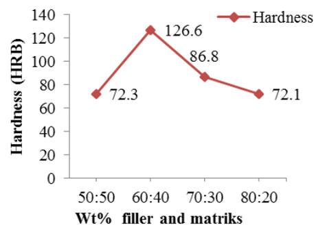
Fig. 7: Variation of hardness wt. % filler and matrix
