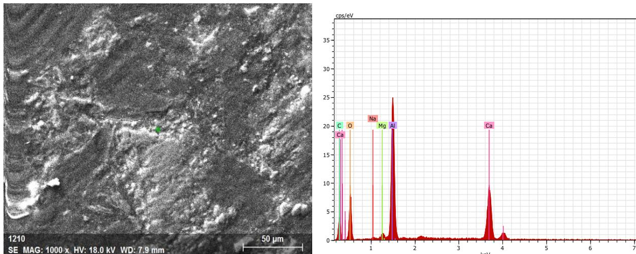
Fig. 26: SEM/EDS Microstructure of developed brake pad with 80 wt. % filler and 20 wt. % matrix
