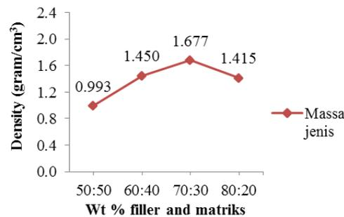
Fig. 5: Variation density with wt % filler and matrix
