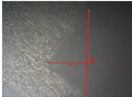
Fig. 20: Wear track depth composition 80 wt. % filler and 20 wt. % matrix (zoom 50 X)
