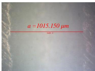
Fig. 15: Wear track width composition 70 wt. % filler and 30 wt. % matrix (zoom 50 X).
