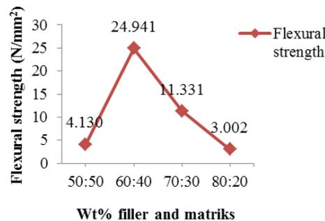
Fig. 6: Variation flexural strength with wt. % filler and matrix.
