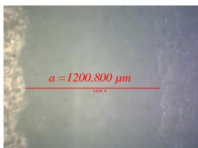
Fig. 16: Wear track width composition 50 wt. % filler and 50 wt. % matrix (zoom 50 X).
