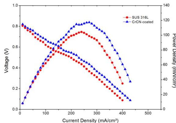
Fig. 13:  $i$ - $V$  curves for the single cell stack; active electrode area = 5  $\text{cm}^2$ ,  $T_{\text{cell}} = \text{RT}$ ,  $\lambda_{\text{H}_2} = 0.5$ ,  $\lambda_{\text{O}_2} = 5$ , and  $P = 1$  atm.
