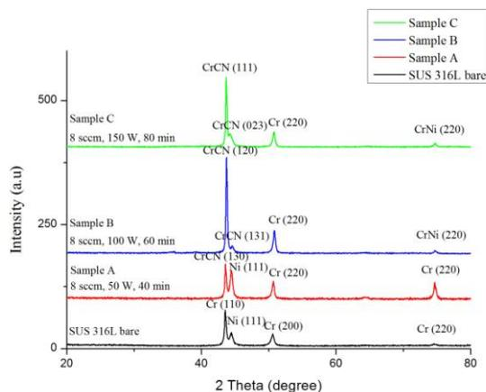
Fig. 4: XRD graph pattern for SUS 316L before and after coating with different CrCN coating parameters.
