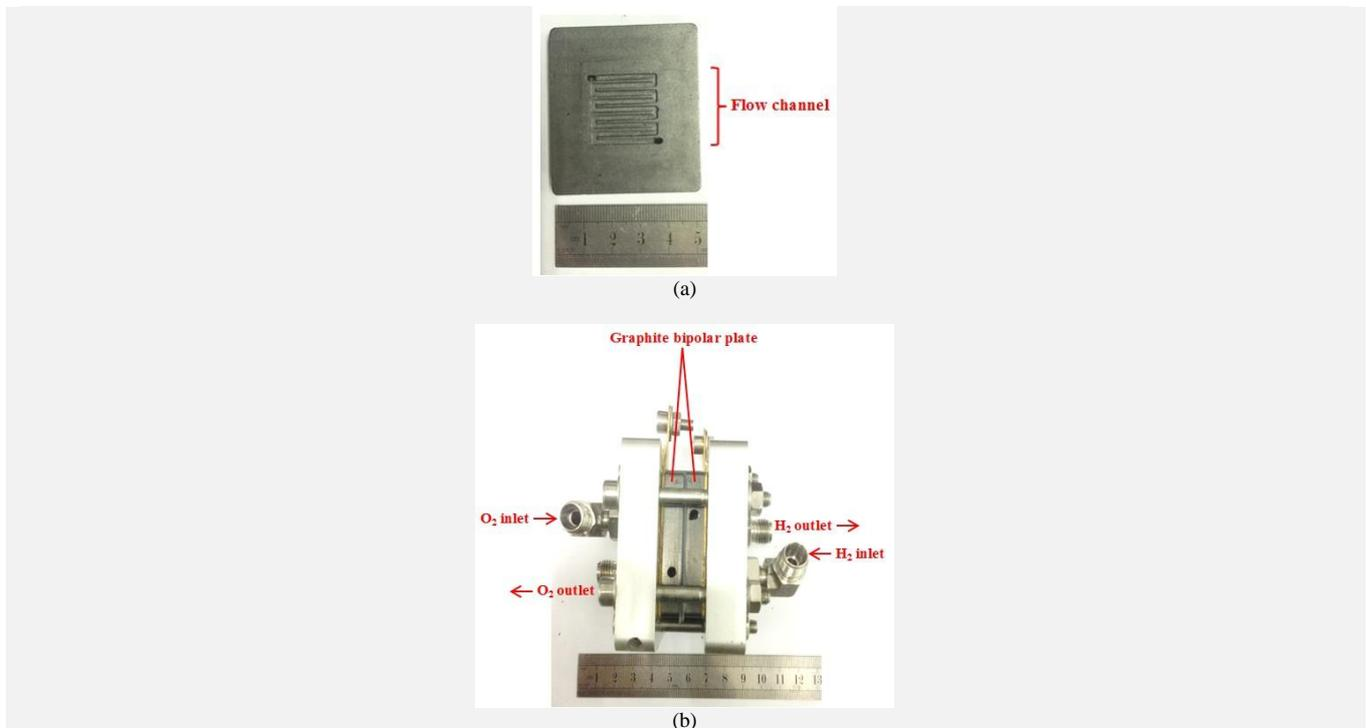
Fig. 3: Bipolar plates made from graphite (a) graphite bipolar plate with serpentine flow channel and (b) single cell bipolar plates.
