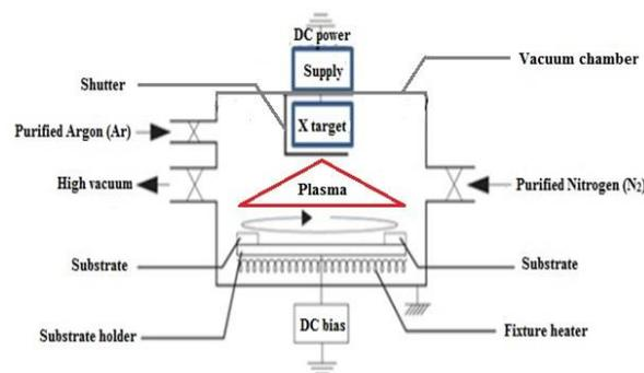
Fig. 1: Schematic assembly of the PVD system [13].
