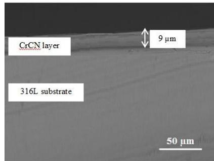
Fig. 12: Cross-section of SEM micrograph image of CrCN-coated SUS 316L for Sample C.
