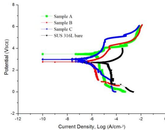
Fig. 7: Polarization curves for uncoated SUS 316L and CrCN-coated SUS 316L in 0.5 M H<sub>2</sub>SO<sub>4</sub>.
