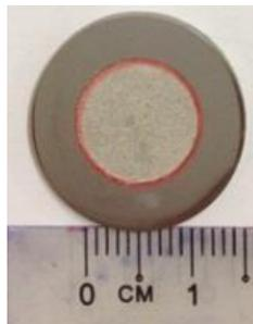
Fig. 8: Macrostructure observation of CrCN-coated for Sample C with 10 mm surface area exposed in 0.5 M  $H_2SO_4$ .
