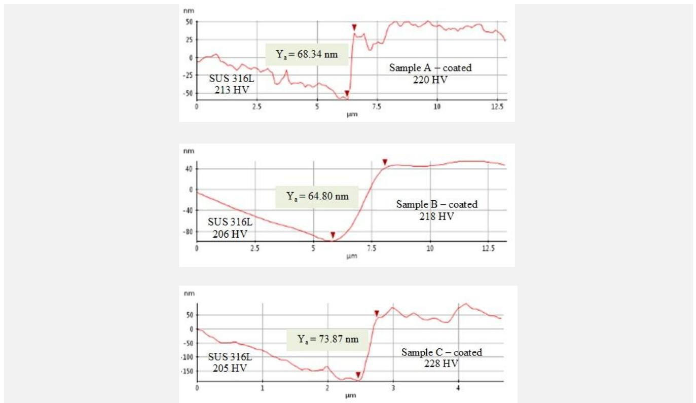
**Fig. 11:** Graph of step height versus distance between CrCN-coated and SUS 316L plates.
