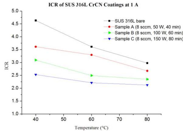
Fig. 6: ICR pattern for SUS 316L with different coating parameters at 1 A.
