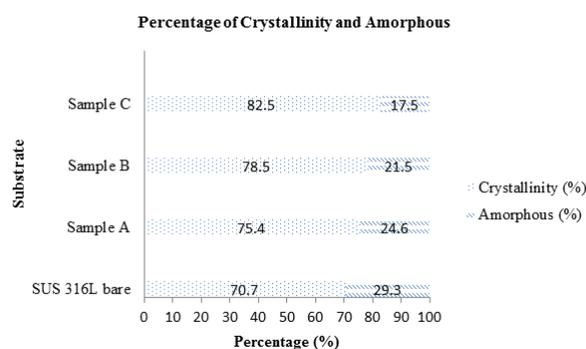
Fig. 5: Percentage of crystallinity and amorphousness of samples before and after CrCN coatings with different parameters.
