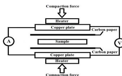
Fig. 2: Schematic of the test assembly for the ICR system.
