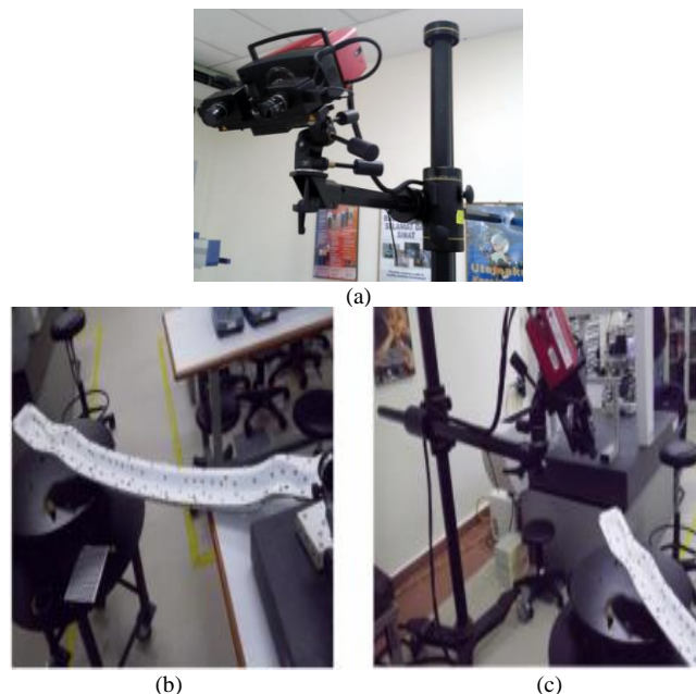
Fig. 2: (a) Three-Dimensional scanner and projector camera (b) Recoloring and reference nodes (c) Scanning process
