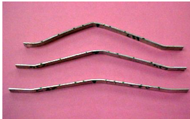
Fig. 4: Tested Beam of 1.55 mm Thickness Arranged in Increasing Order of Impact Velocity from Bottom to Top (17.4 m/s , 24.0 m/s , 27.8 m/s)
