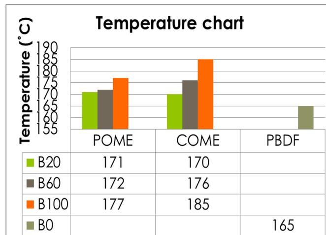
Fig. 5: The graph shows for T<sub>upper</sub> among the blends for COME, POME and PBDF.
