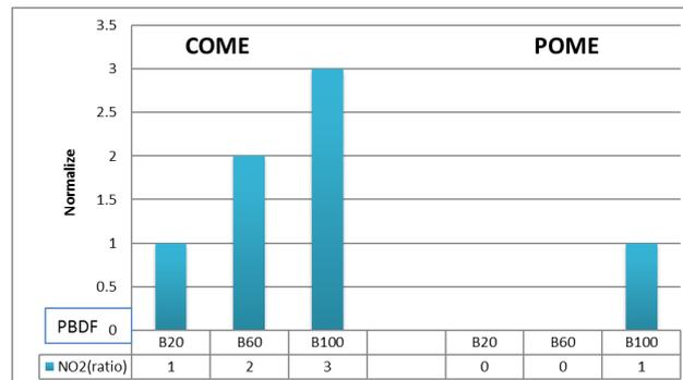
Fig. 4: The graph for COME and POME compare with PBDF in term of NO<sub>2</sub>.
