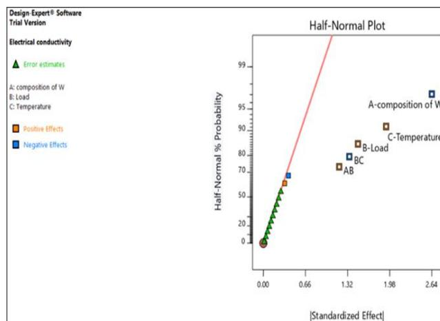
Figure 6: Half-Normal Plot for electrical conductivity
