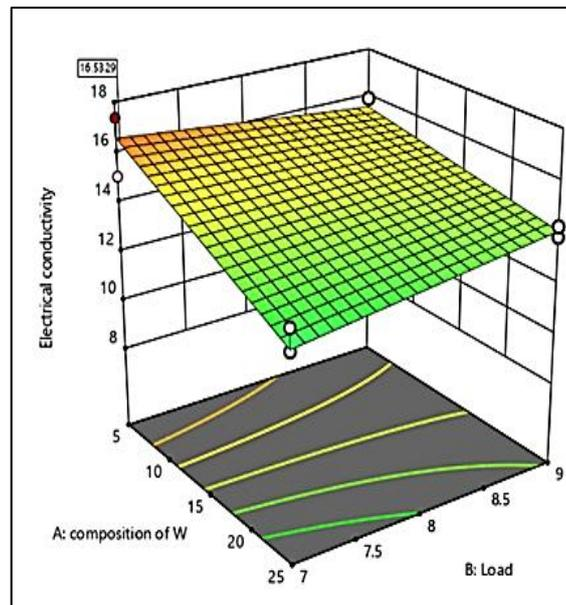
Figure 7: Optimum 3D surface electrical conductivity with the used of 735°C of sintering te
