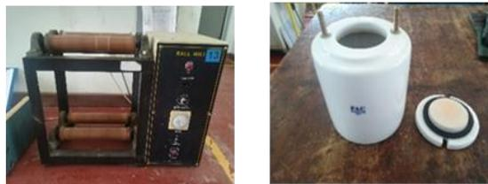
**Figure 2:** Ball milling machine and ceramic beaker
