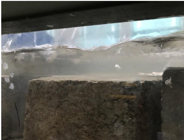
Fig. 3: Sub-Grade Soaks into Water for 24 Hour.
