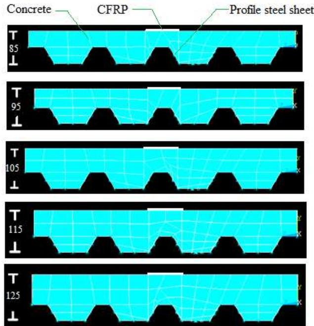
Fig 5: Cross-section of CCS FE models with different slab thicknesses.
