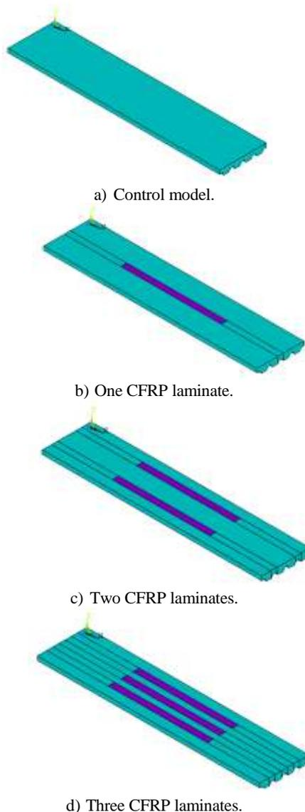
Fig 9: CCS models strengthened with different numbers of CFRP laminates.
