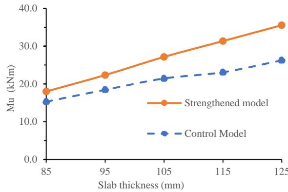
Fig 6: Ultimate moment capacity ( $M_u$ ) of CCS with different overall slab thicknesses.
