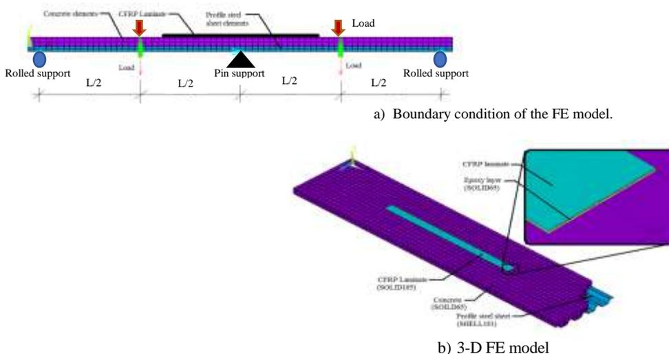
Fig 1: FE modelling of the proposed composite slab system.
