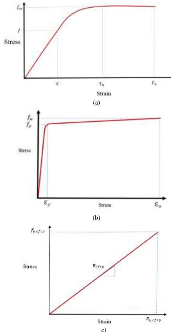
**Fig 2:** Stress-strain relationships of materials; a) Concrete, b) Profiled steel sheet, c) CFRP Laminate
