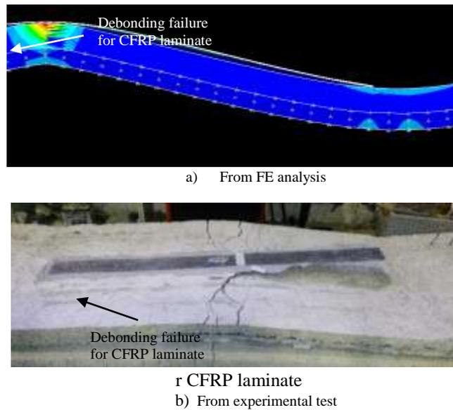
Fig 4: CFRP failure mode for the FE model and experimental specimen CCS-1.7L.
