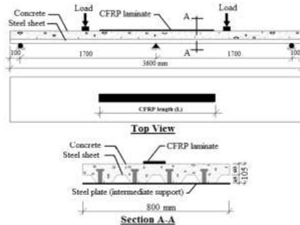
Fig 1: The specimens of the strengthened continuous composite slab (all dimensions in millimetres). [12]
