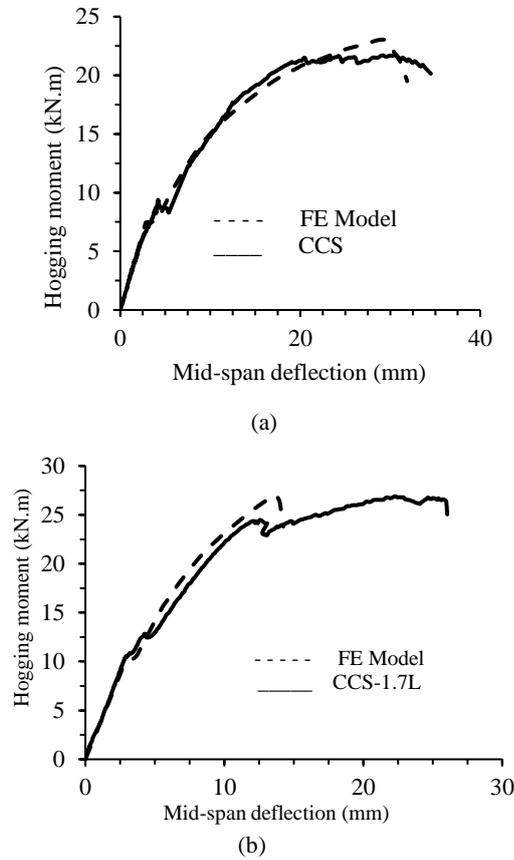
Fig 3: Moment-deflection verification of slab specimens with FE Model; (a) CCS and (b) CCS-1.7L.
