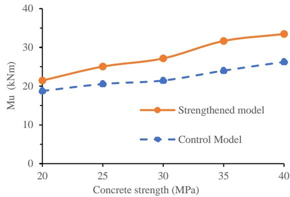
Fig 8: The hogging  $M_u$  of the strengthened CCS model with varying concrete strength.
