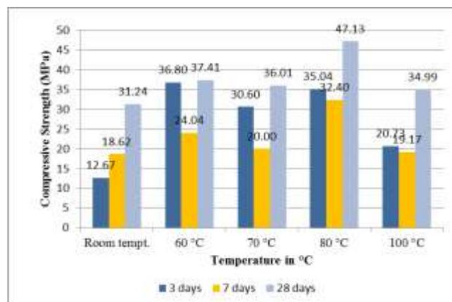
Fig. 2: Effect of Elevated Curing Temperature on Compressive Strength of Geopolymer Concrete at ages 3 days, 7 days and 28 days.
