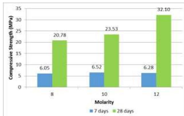
**Fig. 1:** Effect of Molarity of Alkali Solution on Compressive Strength of Geopolymer Concrete. All sample curing under ambient condition.
