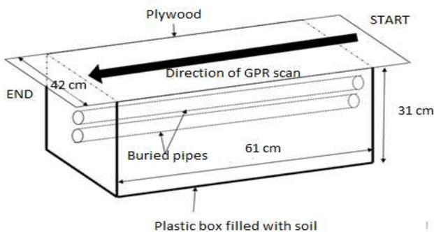
Fig. 1: Schematic diagram of the prototype model
