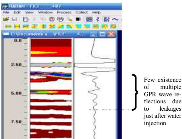
Fig. 4: GPR signal Profile C
