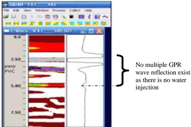
Fig. 2: GPR signal before the water addition (Profile A)
