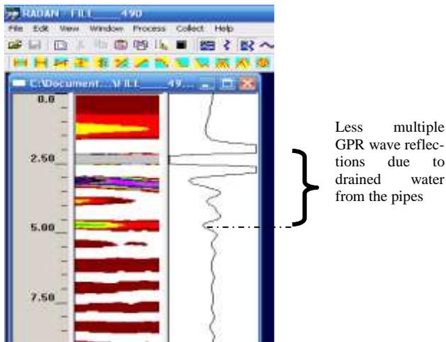
Fig. 5: GPR signal Profile D
