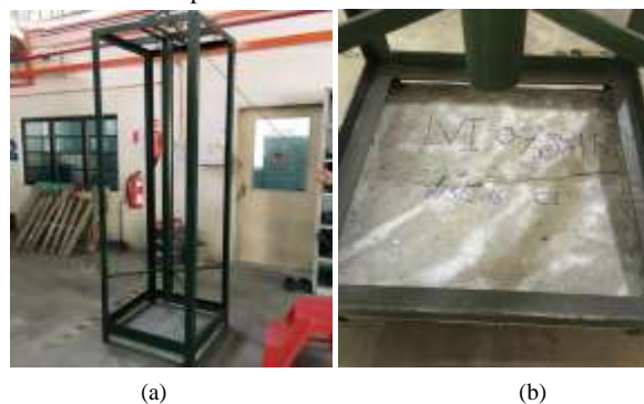
Fig. 2: a) Low velocity impact test Frame .b) crack form of Specimen installed in frame
