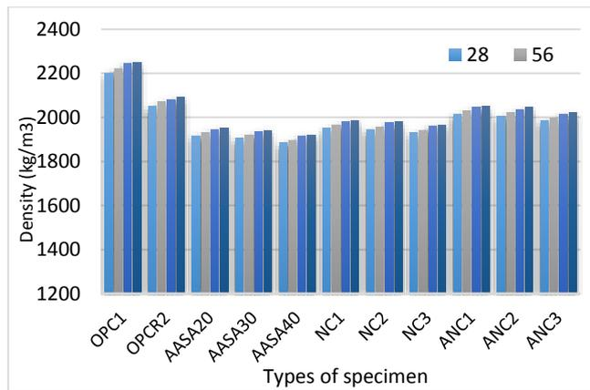
Fig. 1: Bulk density of specimens
