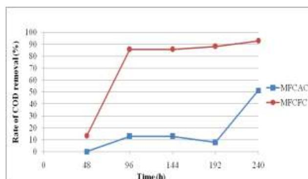
Fig.4: COD removal efficiency over time
