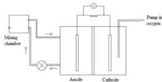
Fig.1: Self fabricated reactor.
