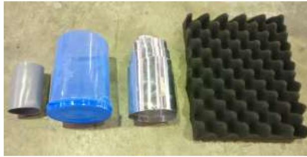
**Fig. 3:** Acoustic shield adopted in testing. From left, PVC pipe, PP plastic, aluminium sheet and egg crate foam.
