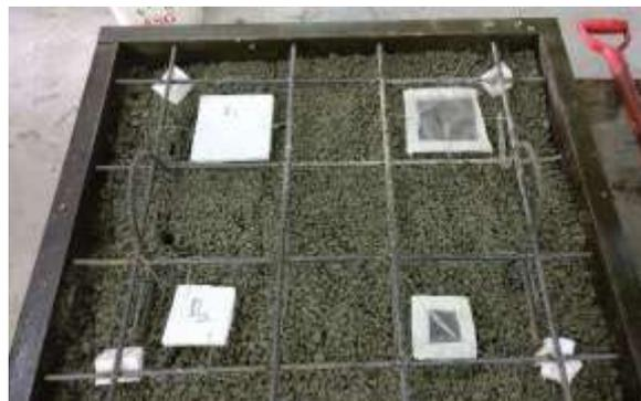
Fig. 2: Placement of artificial defects during sample preparation.
