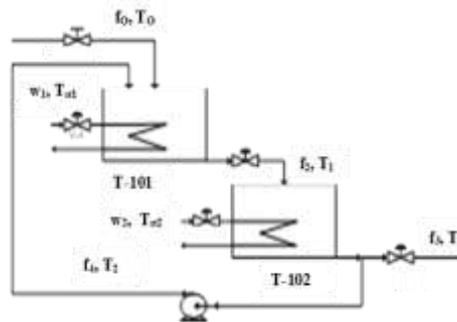
Fig. 1: Two Stirred Tank Heat Exchanger in Series
