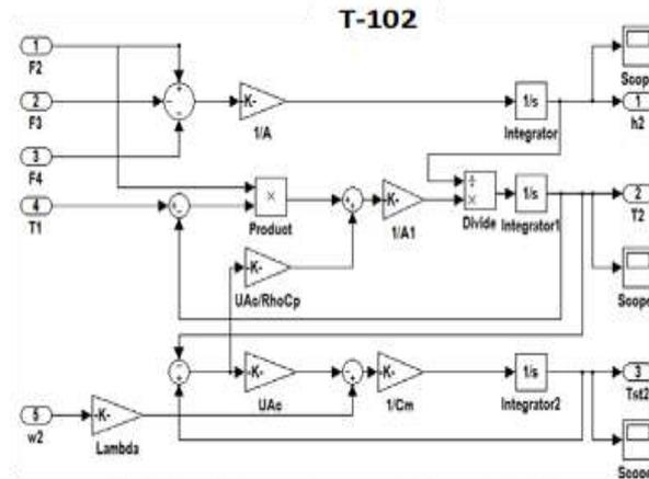
Fig.3: Simulink open-loop model for tank T-102
