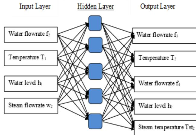
Fig. 6: MLFFN network for T-102 at dynamic state
