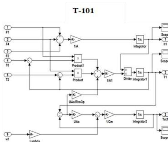
Fig 2: Simulink open-loop model for tank T-101
