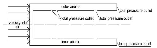
Fig. 3: Flipchart Shows the Boundary conditions in CFD
