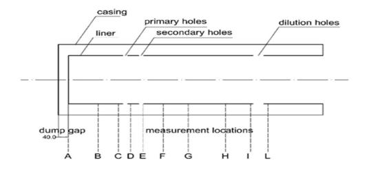
Fig. 1: Can Combustor Layout
