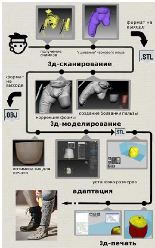
Figure 1: Diagram of the technique of applying 3D printing technology in lower limb prosthetics
