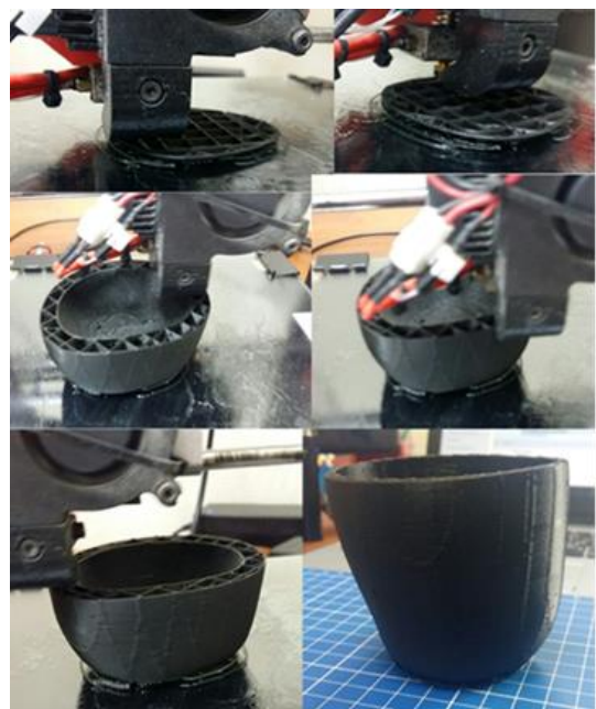
Figure 3: Stages of 3D printing of a culture receiving sleeve
