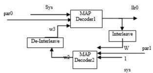
Fig. 3: Block Diagram of Turbo Decoder. Using Map Algorithm.
