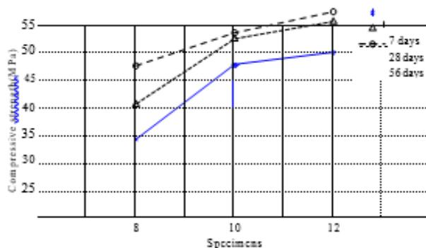
Fig. 3: Variation of Compression Test with Fiber Fraction.
