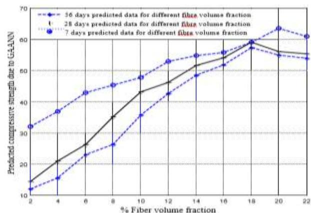
Fig. 6: Variation of Predicted Compressive Strengths of Proposed ANN with Fiber Volume Fraction.
