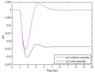
Fig.3.4: Step Responses of HOS and LOM Without Controller and with Controller.
