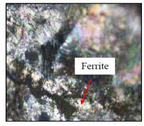
Fig. 3: The microstructure of an as-cast niobium alloyed grey cast iron
