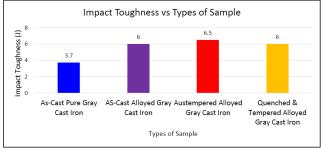
Fig 11: Impact toughness of different types of specimens
