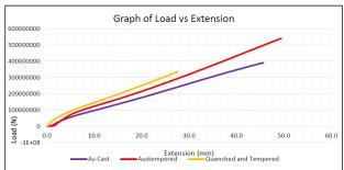
Fig. 10: Relationship between load and extension of different types of specimens
