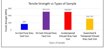
Fig. 8: Tensile strength of various types of specimens
