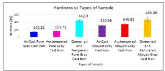
Fig. 7: Hardness of various types of specimens
