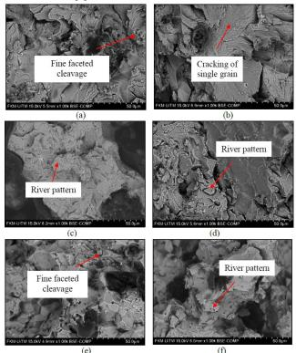
**Fig 12:** S.E.M. Observations at Magnification of x1000 (a) As-cast Alloyed (Tensile), (b) As-cast Alloyed (Impact) (c) Austempered Alloyed (Tensile), (d) Austempered Alloyed (Impact) (e) Q&T (Tensile), (f) Q&T (Impact)
