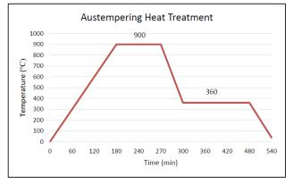
Fig. 1: Schematic diagram of austempering heat treatment
