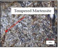
Fig. 6: Structure of tempered martensite
