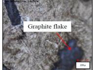
Fig. 5: The structure of graphite flake in grey cast iron
