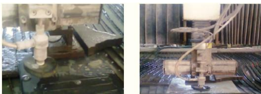
Fig.1: Carbon Fiber Reinforced Composite Laminate & Glass Fiber Reinforced Composite Laminate Cutting Process.
