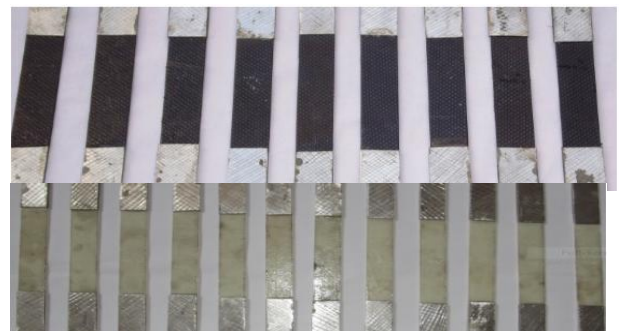
Fig.3: Untested Coupons of CFRP and GFRP (Without Damage)
