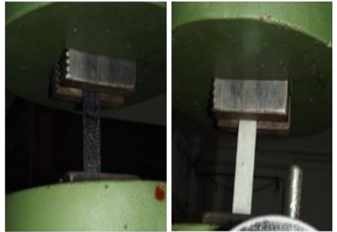
Fig. 6(b): UTM testing damaged coupon
