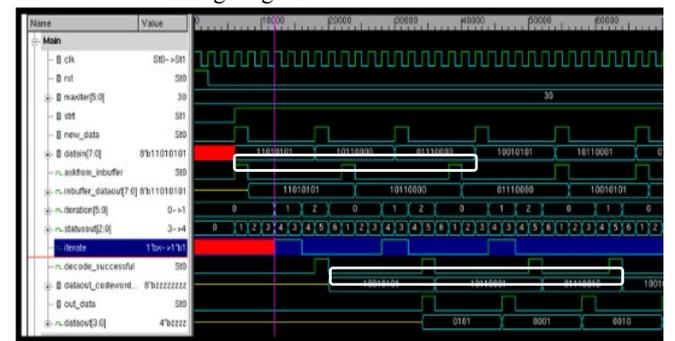
Fig. 9. Main LDPC\_decoder module timing diagram
