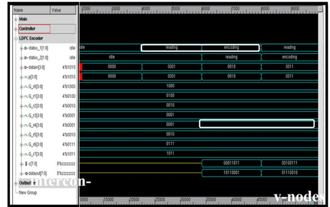
Fig. 7. LDPC\_encoder module timing diagram
