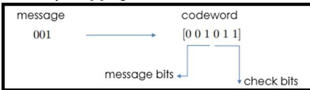
Fig. 1. The Message, check, and code word bits in an FEC encoded message
