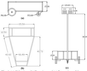
Fig. 1. (a) Side view, (b) Top view and (c) Front view of the cart
