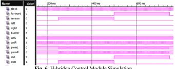
Fig. 6. H-bridge Control Module Simulation
