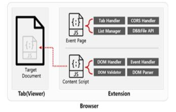
Fig. 2 Structure of collector-based browser extension
