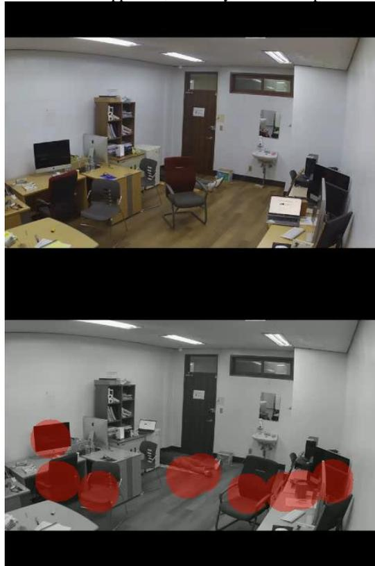
Fig. 13: Indoor object detection using our vision classifier (upper one: raw camera image, lower one: frequently used furniture)
