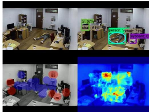
Fig. 16: Unusual stationary behavior in an infrequent location and detection using our vision classifier.
