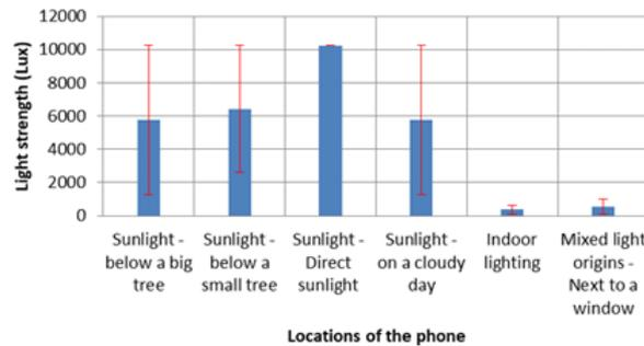
Fig. 18: Experiment using a Light sensor on the HTC Sensation
