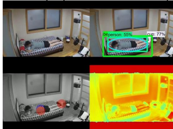
Fig. 15: Normal stationary behavior on the bed and detection using our vision classifier
