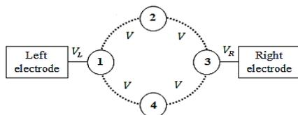
**Fig 1:** Schematic diagrams of quantum dot ring connected with two electrodes.
