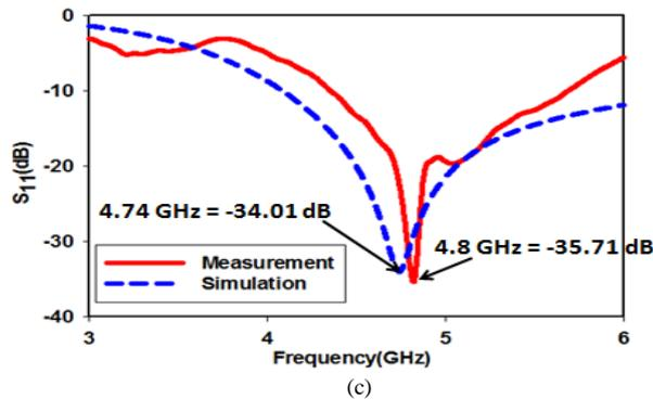
Fig. 4: Simulated and measured reflection coefficient,  $S_{11}$  of cylindrical monopole plasma antenna. (a) Argon gas. (b) Neon gas (c) Hg-Ar gas
