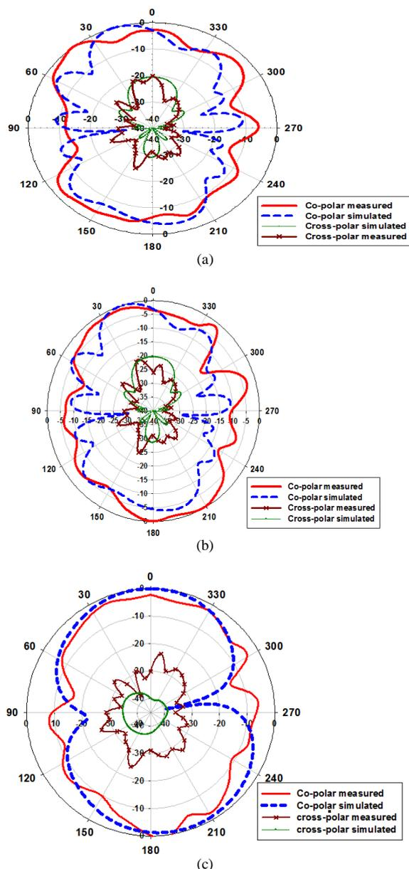
Fig. 5: Simulated and measured radiation patterns. (a) Argon gas (b) Neon gas (c) Hg-Ar gas
