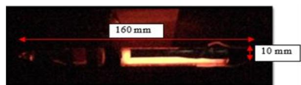
Fig. 1: Cylindrical monopole plasma discharge tube.
