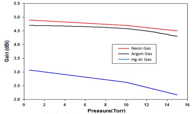
Fig.3: Effect in gain for different pressure
