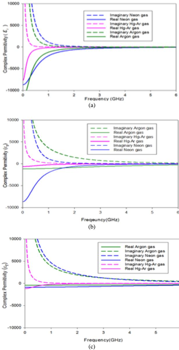
Fig. 2: Relative Permittivity for argon gas, neon gas and Hg-Ar gas for (a) 0.5 Torr (b) 5 Torr and (c) 15 Torr.
