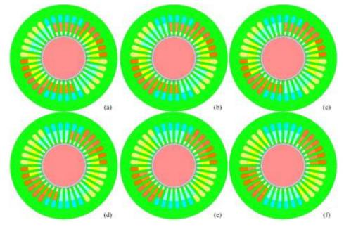
Figure 2: Structure of high-speed PMSG according to winding distribution: (a) coil pitch 13, (b) coil pitch 14, (c) coil pitch 15, (d) coil pitch 16, (e) coil pitch 17, (f) coil pitch 18
