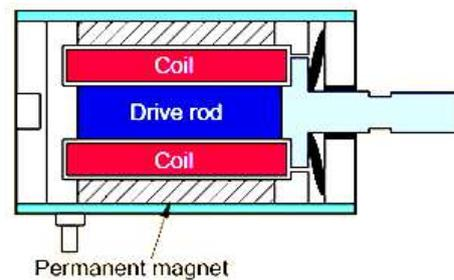
Figure 3: Type of Vibrator according to Vibration generation method
