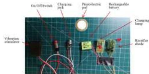
Figure 7: Electronic devices for Manufacturing Vibration stimulators
