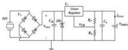
Figure 4: Power Charging circuit of Vibration stimulator using Bridge circuit
