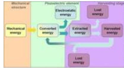
Figure 2: Concept of Energy harvesting process using Piezoelectric element
