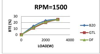
Fig: 3: Variation of BTE with load
