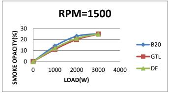
Fig: 9: Variation of Smoke with Load
