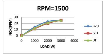
Fig: 7: Variation of NOx with Load
