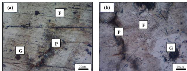
**Fig. 4:** Microstructure of Ductile Iron at 500 Times Magnification: (a) 0.1g/L Inhibitor Concentration (b) 0.3g/L Inhibitor Concentration. G: Graphite Nodule; F: Ferrite; P: Pearlite
