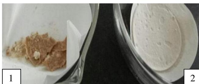
Fig. 1: CAMC before [1] and after wash [2]
