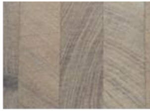
Fig. 1: Glulam made of Mengkulang species
