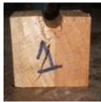
Fig. 8: Typical cracks for specimen with glue line
