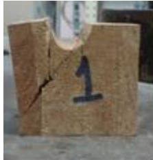
Fig. 9: Typical cracks for specimen without glue line
