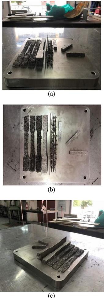
**Fig. 5:** Printed specimens from SLM process: (a) front view, (b) top view, and (c) isometric view
