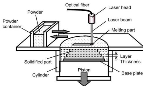
Fig. 1: Experimental equipment for selective laser melting process.
