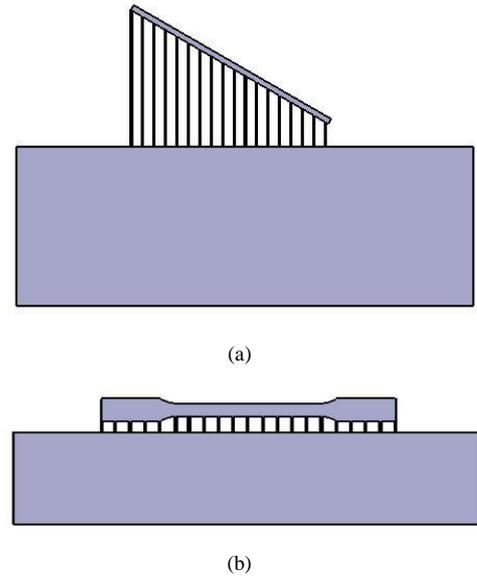
**Fig. 7:** (a) Sample D3; horizontal build direction, (b) Sample T3; vertical build direction.
