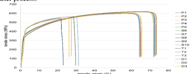
Fig. 4: Tensile test for each specimens from SLM and rolling process
