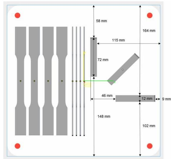
Fig 3: Dimension of the substrate plate.
