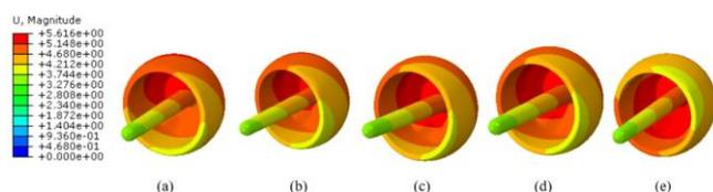
**Fig. 8:** Deformation of hip resurfacing femoral component during normal walking conditions. (a) Straight, (b) Varus  $-5^\circ$ , (c) Varus  $+5^\circ$ , (d) Sagittal  $+5^\circ$ , (e) Sagittal  $-5^\circ$
