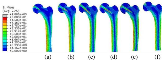
Fig. 4: Von misses stress of HRA models during normal walking conditions, (a)varus -5°, (b)straight, (c)varus +5°, (d)sagittal +5°, (e) sagittal -5°, (f) half femur
