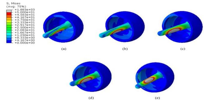
Fig. 6: Von misses stress of RHA femoral component for normal walking condition, (a)straight, (b)varus -5°, (c)varus +5°, (d)sagittal +5°, (e)sagittal -5°
