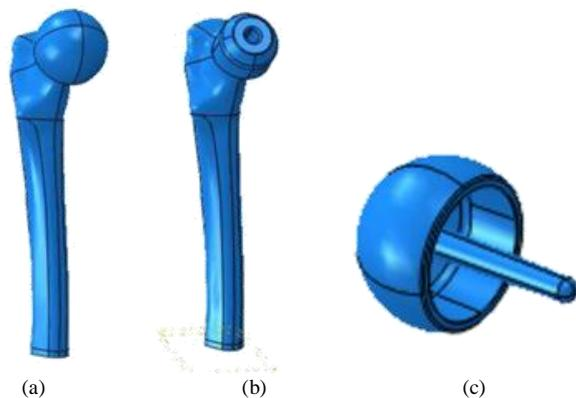
Fig. 1: 3D model of (a) half femur, (b) femur component, (c) femoral component
