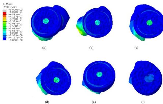
Fig. 5: Von misses stress of RHA models and half femur on the cross-section of the proximal region for normal walking condition, (a)straight, (b)varus +5, (c)varus -5d) sagittal +5, (e)sagittal-5, (f) half femur
