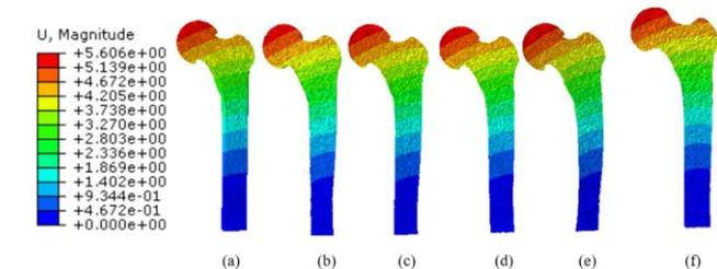
Fig. 7: Deformation of hip resurfacing femoral component during normal walking conditions, (a) Straight, (b) Varus -5°, (c) Varus +5°, (d) Sagittal +5°, (e) Sagittal -5°
