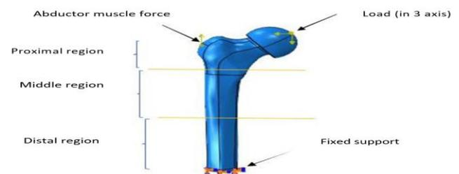
Fig. 3: An illustration of the loading conditions of the HRA model for normal walking.
