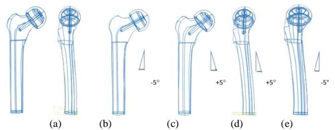
Fig. 2: Different type of malalignment, (a) neutrally aligned 125°, (b) varus -5°, (c) varus +5°, (d) sagittal flexed +5°, and (e) sagittal extended -5°.
