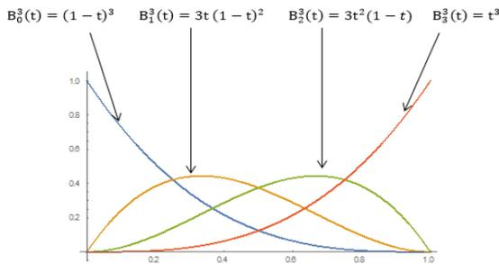
Fig 3: The Cubic Bezier basis
