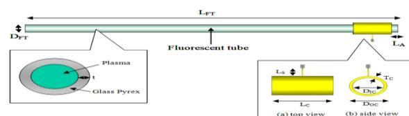
Fig. 1: Geometry of the monopole plasma antenna
