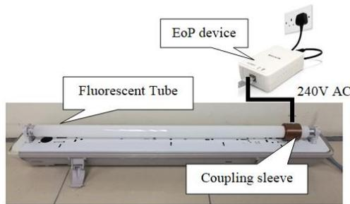
**Fig. 3:** Monopole plasma antenna with EoP device
