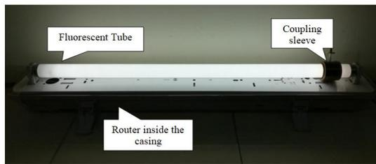
**Fig. 2:** Monopole plasma antenna with Wi-Fi router
