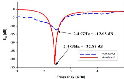
Fig. 5: The comparison of  $S_{11}$  between simulated and measured result.
