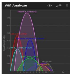
Fig. 7: Performance of signal strength of monopole plasma antenna
